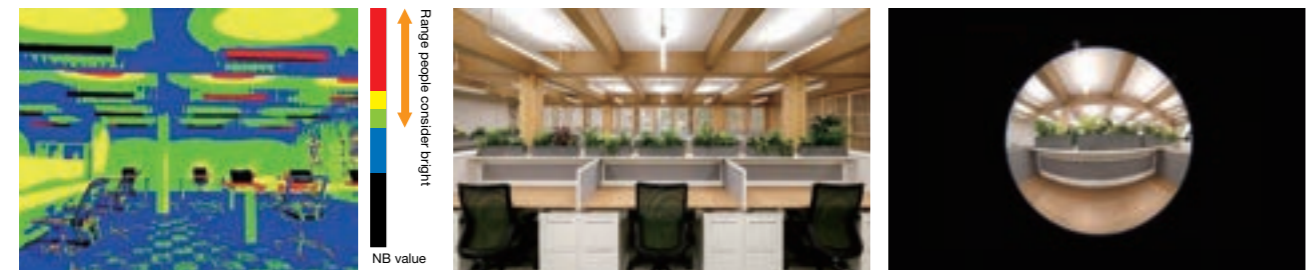
At the design stage, we use simulations to study the brightness of a space. We can achieve a bright environment even in low-energy buildings like ZEBs.
