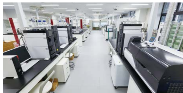
Row of Shimadzu Liquid Chromatograph Mass Spectrometer Systems at the Bacchus Laboratory
