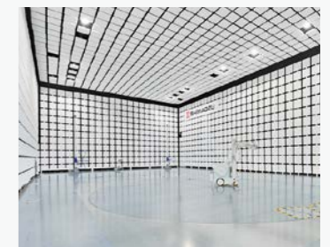
Quality Center's 10-Meter Method Anechoic Chamber
