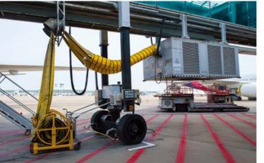
AC-GPS supplies power from the ground while the aircraft is on the ground. It reduces carbon emissions by not running the APU (auxiliary power unit).
