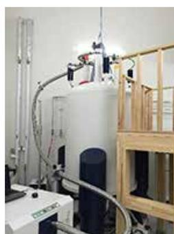
800 MHz superconducting nuclear magnetic resonance equipment
