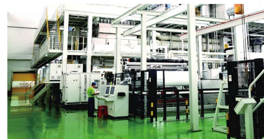
◆ New high-speed "Hongda V-type" complete equipment for spun-melt nonwovens built by Hongda Institute, SINOMACH.
