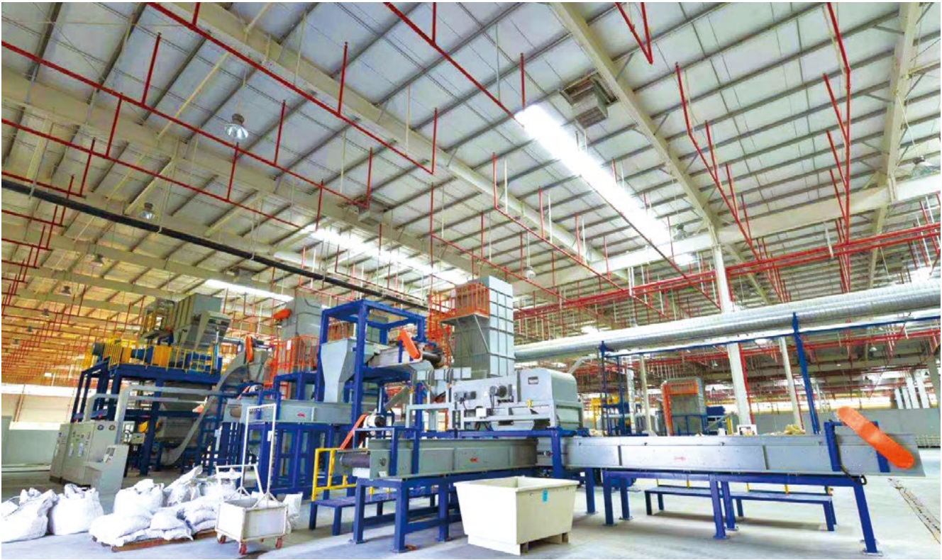
◆ The production line for eliminated refrigerator recycling developed by CEI
