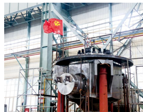
◆ SINOMACH HE's automatic weld overlay technology for the inner wall of the third-generation nuclear power pump.
