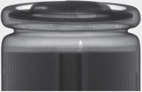
X-ray image of lithium-ion rechargeable battery designed for electric vehicle use
