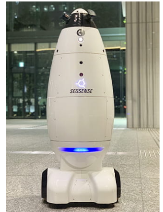
Security robot SQ-2 (Otemachi Park Building) Replacing human patrols and guards through advanced autonomous movement functions
