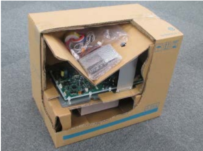
Internal structure of the revamped packaging
