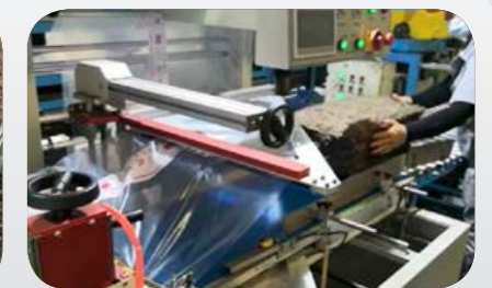
Technology-Innovation: Automated rubber bale-wrapping process in China to improve operational safety
