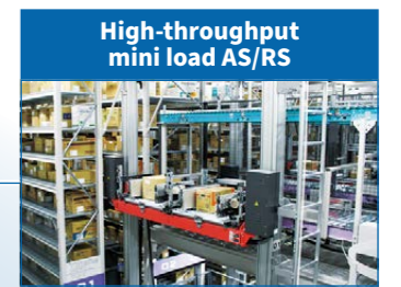
Stores various-sized cardboard boxes and facilitates case shipping
