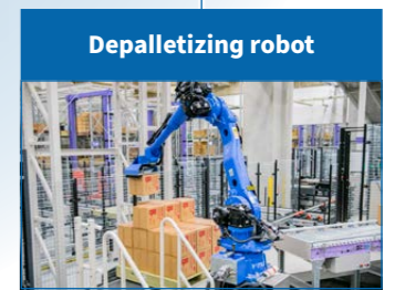
Picks cardboard boxes from a pallet retrieved from an AS/RS
