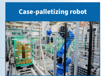
Rapidly palletizes cases of various shapes and sizes
