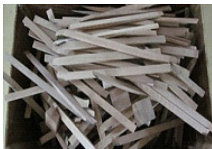
Timber offcuts previously disposed of as waste being repurposed as corner block (structural reinforcement materials inside guitar bodies)
