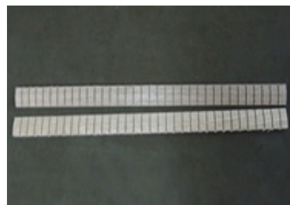
Timber offcuts previously disposed of as waste being repurposed as corner block (structural reinforcement materials inside guitar bodies)
