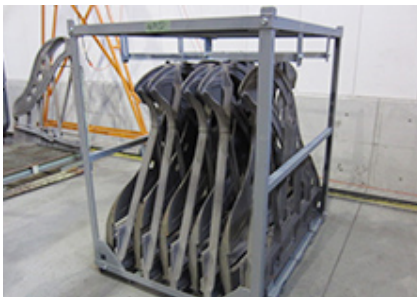
Returnable packing rack for grand piano frames
