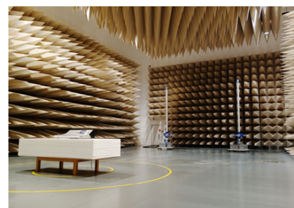
Anechoic chamber used for electromagnetic wave measurement
