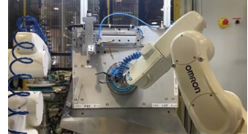
Two OMRON robots shaping blue polyurethane circle parts
