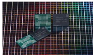
176-layer 4D NAND based 512Gb TLC that SK hynix invented
