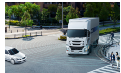
Blind spot monitor that projects from the cab in four directions
