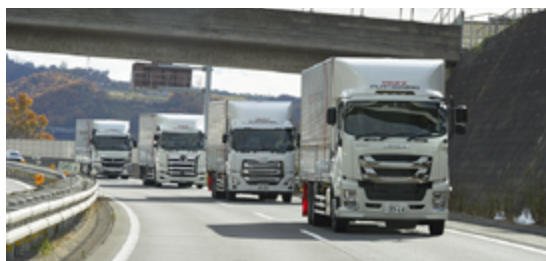
Highway validation test for truck platooning
