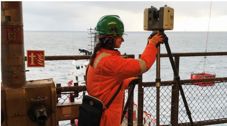
Magda Oglodek of GDi laser-scanning the Bruce Platform for the digital twin
