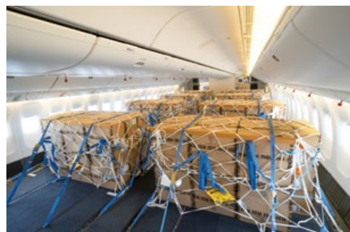
Modification of the Aircraft to Accommodate Cabin Floor Loading
