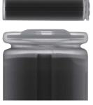
Internal shape inspection of Li-ion batteries
