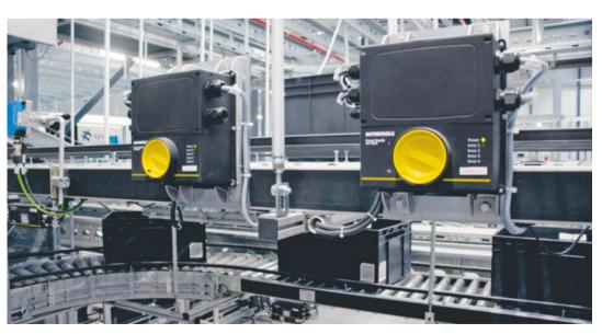
Efficient power supply: The robust, ready-to-use switched-mode power supplies with IP54 degree of protection are mounted directly where the protective extra-low voltage is needed, and not in the control cabinet. This allows much shorter cable lengths. The result is very short cables, which reduce power and and material consumption and reduce faults such as a possible drop in line voltage, as well as a positive contribution to occupational safety.
