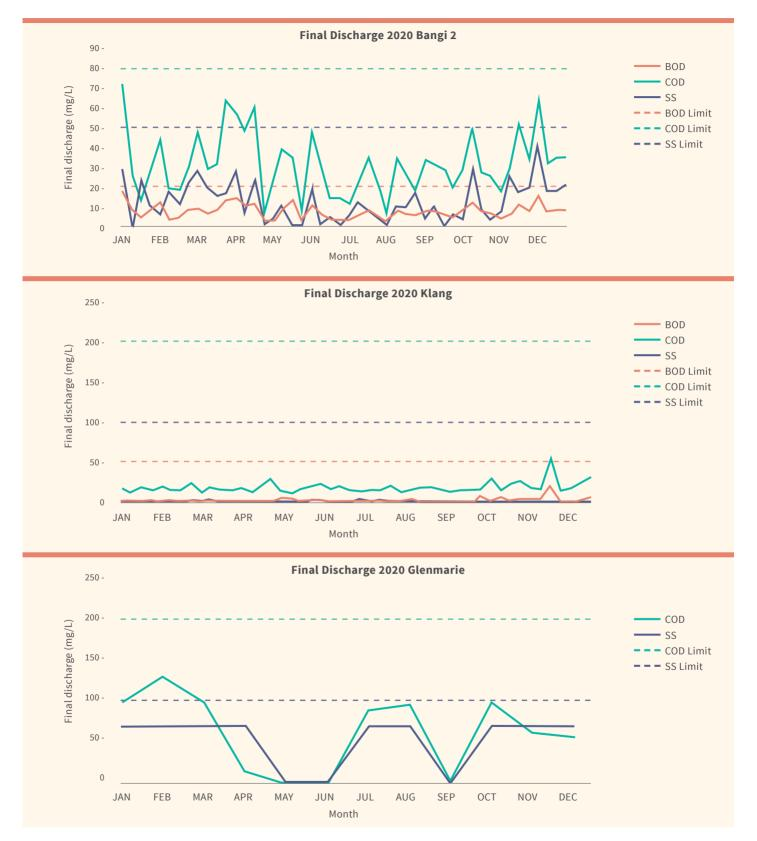
Monthly discharge at Glenmarie fluctuates widely because effluents are treated only when a certain volume is collected, as opposed to continuously. Because of the batch method used, the COD limit for Glenmarie is 200mg/L. For the year, all our plants met the relevant regulatory limits for effluent discharge.
