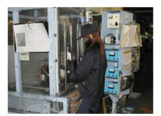
2. Gas leak inspection After ensuring there are no leaks, refrigerant is sealed inside and a refrigerant detector is used to inspect all brazed parts.
