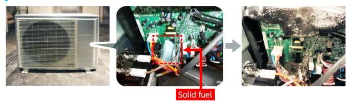
A fire is set on purpose by igniting a point, such as solid fuel or nichrome wire, in a part where risk of fire exists (such as inside the product casing). This is to ensure fire does not spread beyond the product.
