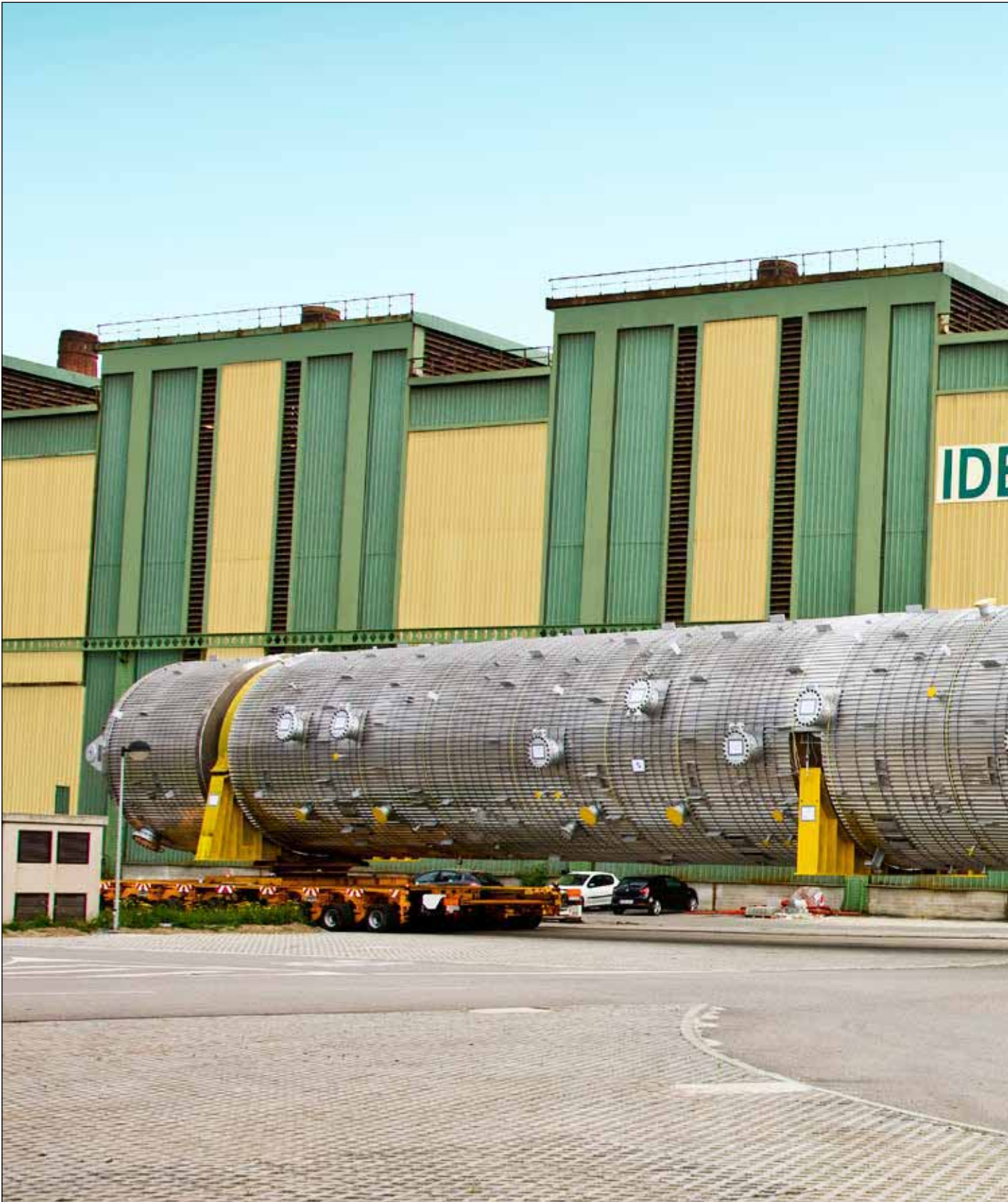
Crude oil secondary column made of stainless steel supplied by Acerinox for the petrochemical industry
