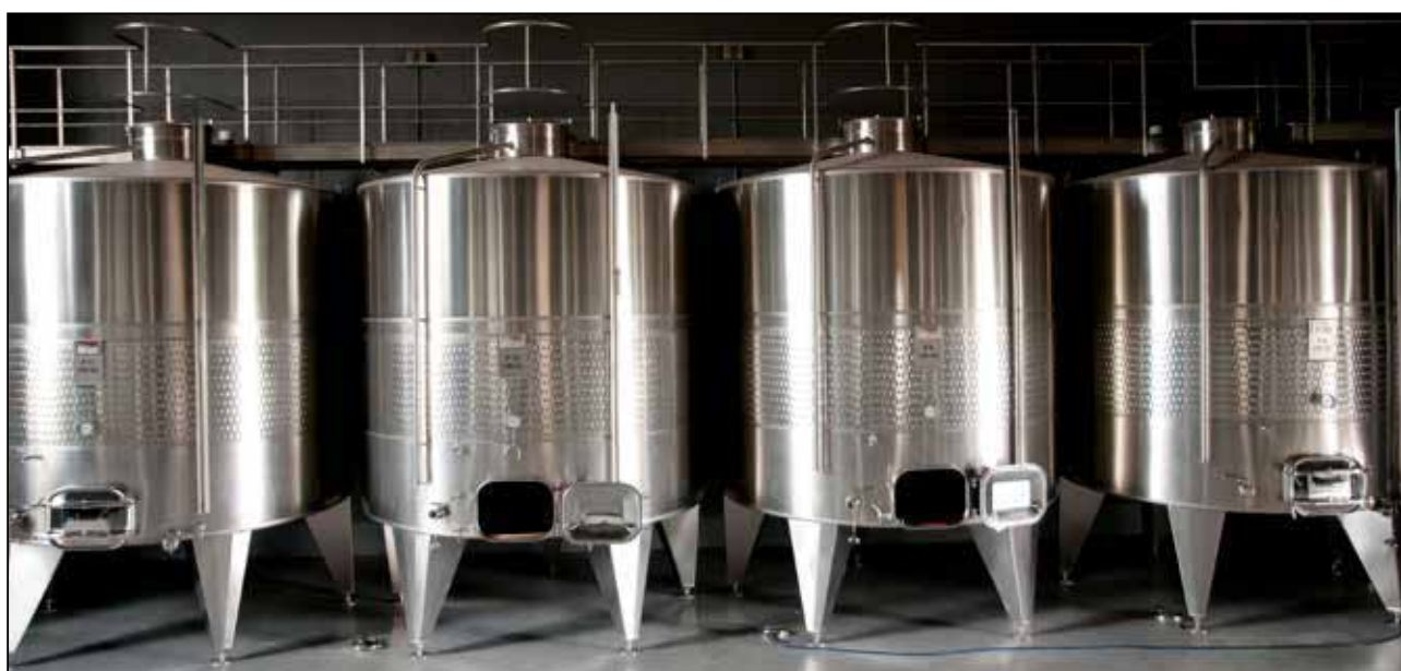
Stainless steel decantation tanks for wine industry
