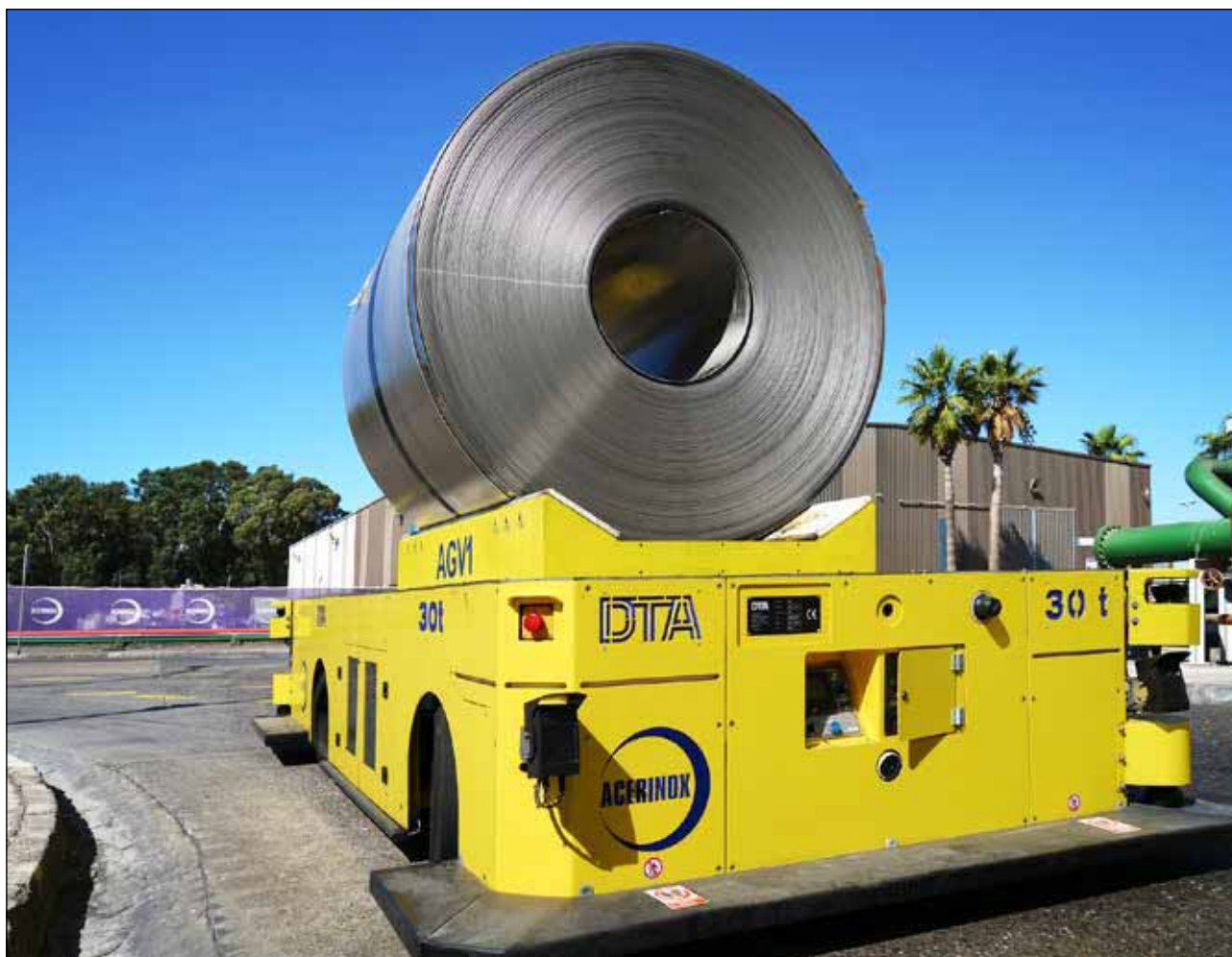
Autonomous guided vehicle for transporting in the Campo de Gibraltar factory (Spain)
