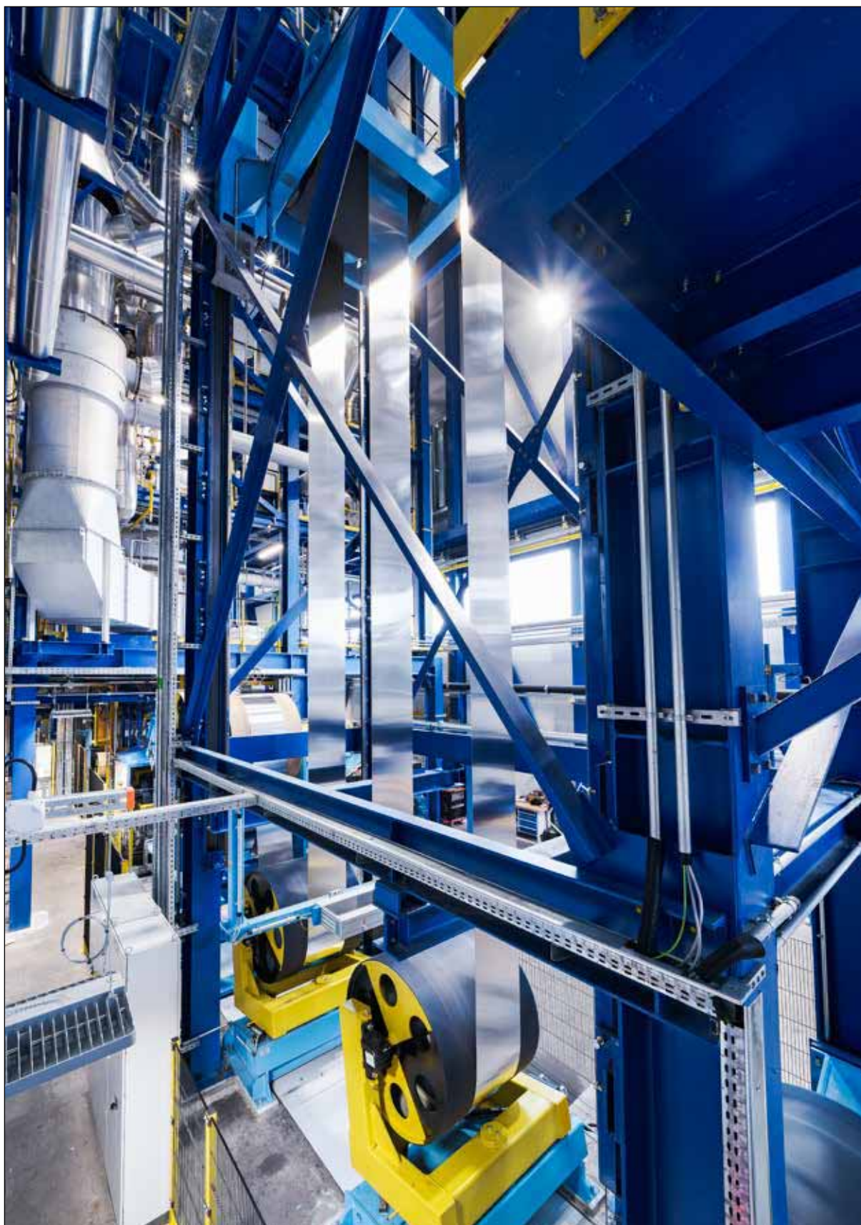
Bright annealing line at VDM
