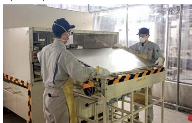
■ CIS thin-film solar cell modules processed by a panel separator
