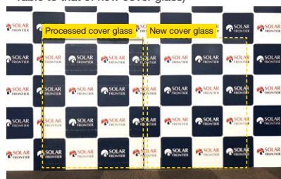
■ Comparison of cover glass processed by a panel separator and the cover glass of a new solar panel (Transparency of processed cover glass is comparable to that of new cover glass)
