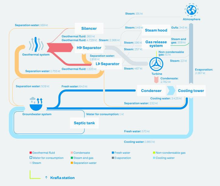
The main flow of steam is through the turbines of the station where the electricity generation takes place. From there, the steam is released into a condenser and then a cooling tower before being released into the atmosphere. Part of the geothermal fluid is sent into a low-pressure separator, but steam also enters the turbine from the separator.
