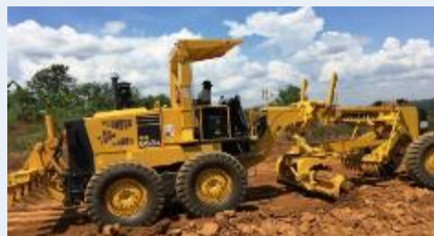
Training of local operators of supplied machines The vehicle in the photo is a motor grader used for ground leveling.
