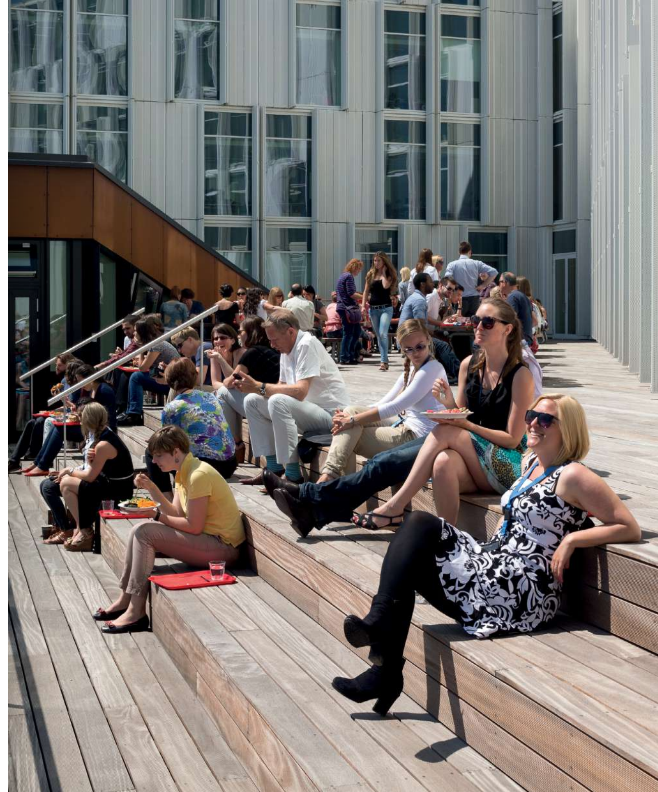
View of the UN City, the headquarters of 11 UN agencies in Copenhagen (Denmark). Here, Tali ( Erythrophleum spp. ), a heavy species of African timber (approx. 900 kg/m 3 ) and known for its resistance to the elements and insects, shines on the beautiful terraces surrounding the building. Designed by Danish architects 3xn, this large building is one of the most energy efficient in Denmark. It has won the European Commission's Green Building Award as well as LEED Platinum certification.
