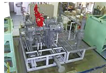
Testing seismic resistance with a 3D shaking table
