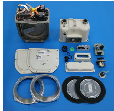
Disassembled gas meter
