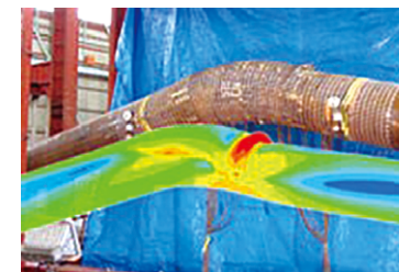
Pipeline deformation behavior assessment using numerical analysis
