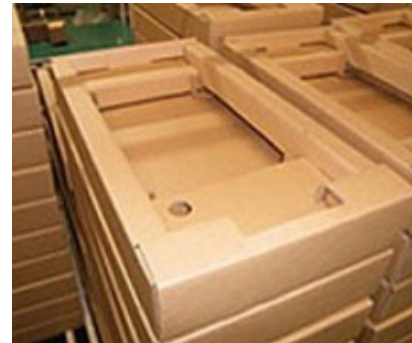
Cardboard boxes designed to require less cushioning
