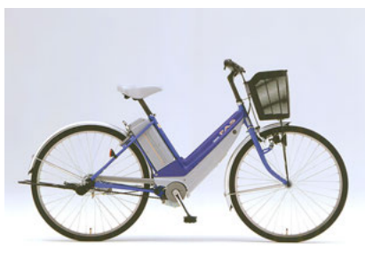
PAS, the world's first electrically power assisted bicycle (1993)
