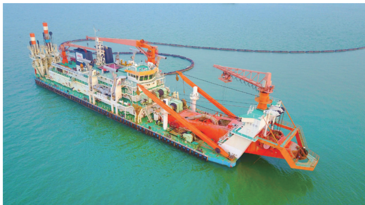
► “铁建绞01”绞吸式挖泥船 Cutter section dredger “CRCC Cutter 01”
