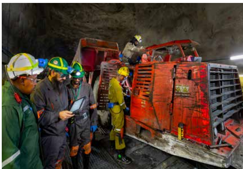
Data from an LHD is downloaded for analysis on a tablet in the workshop at Styldrif
