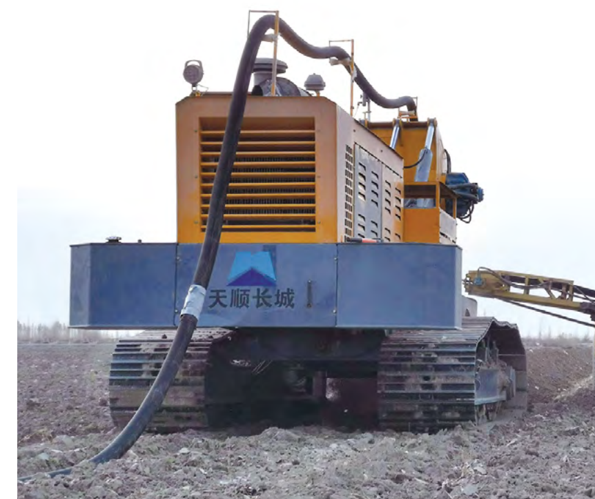
◆ High-power subsurface pipe drainage equipment for saline soil reclamation developed by China Academy of Agricultural Mechanization Sciences (CAAMS), SINOMACH
