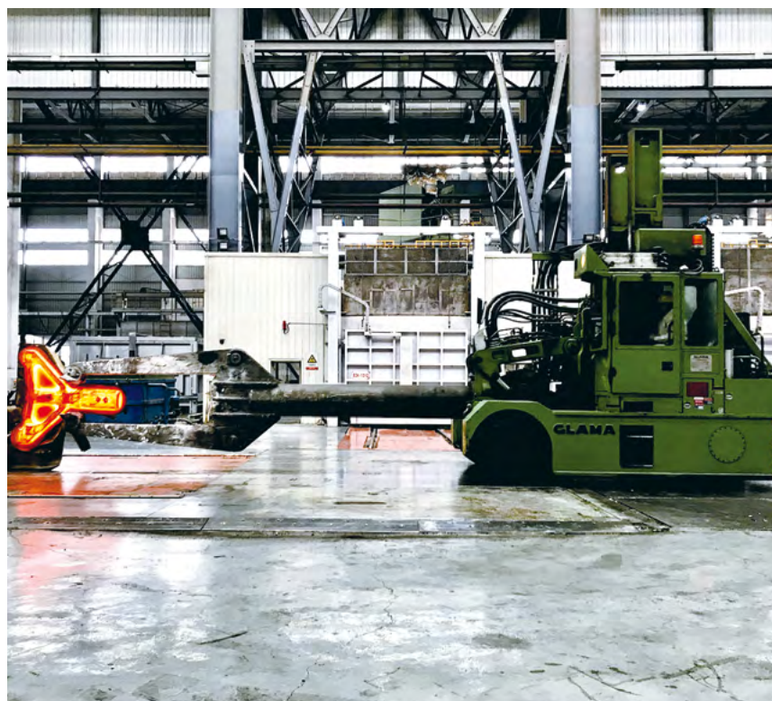
◆ Forging piece of the outer cylinder of the landing gear for Boeing 787 Dreamliner developed by CNEG, SINOMACH
