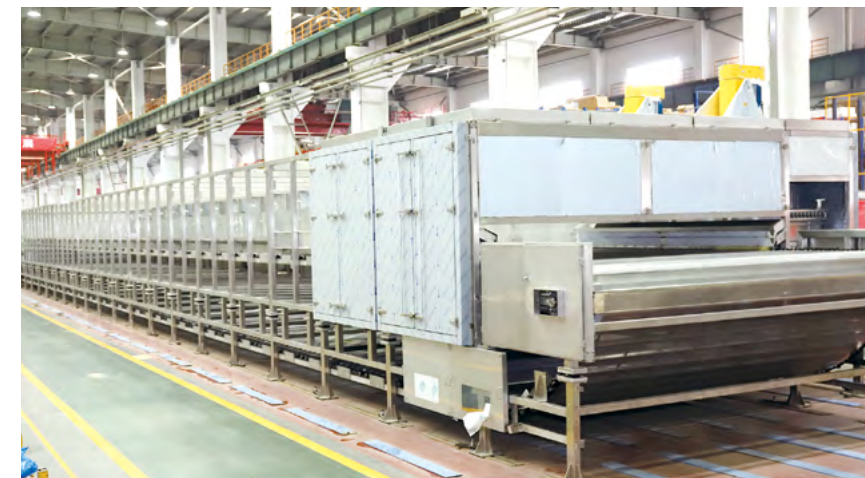
◆ The 15-ton viscose fiber dryer developed by China HiTech Group Corporation (CHTC), SINOMACH
