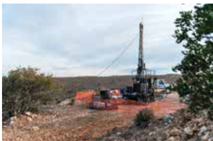
Diamond drill rig in the Fresnillo district
