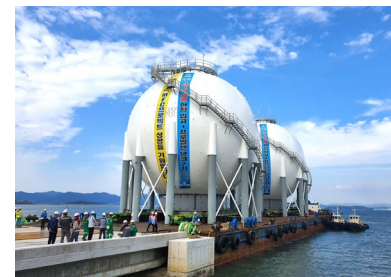
Transportation of Propylene Tank
