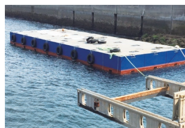
Modular barge system used as a river flood countermeasure (assembled marine construction machinery capable of smoothly performing civil engineering work on water)
