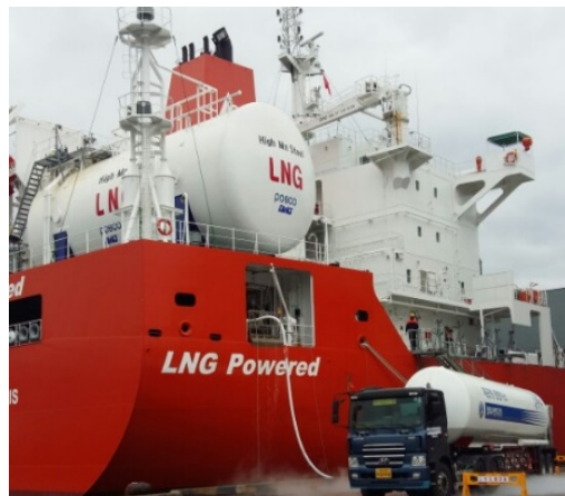
The Green Iris doing bunkering (truck-to-ship)
