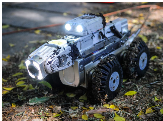
Robot car inspects pipes in search of cracks, infiltrations and obstructions
