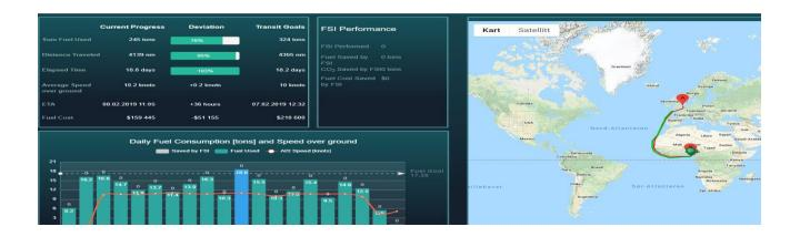
Maress is closely monitored by vessel technical managers and operation department to discover any deviances towards expected consumption/emission with focus in improving efficiency, i.e. reduce consumption/emission. System allows to compare towards set baseline, previous periods (months/years) and between vessels and between shifts on one vessel.
