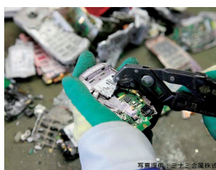
Dismantling of collected mobile phones
