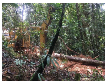
Timber collection using a winch
