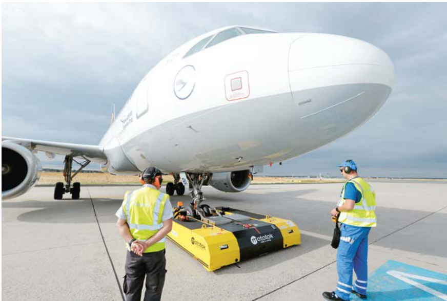
Up to 50 pushback operations are possible with the remote-controlled electric aircraft tow tractor without having to recharge.
