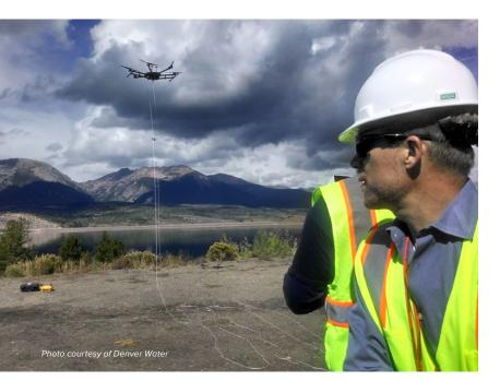
Pit lake water sampling using drone technology
