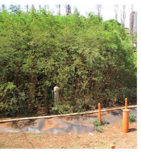
The pilot-scale test ran for two years, proving the idea successful. The trees were found to be effective in remediating the contaminated soil and groundwater. Soil contaminant concentrations were reduced to be below residential standards. and leachate water below drinking water standards.
