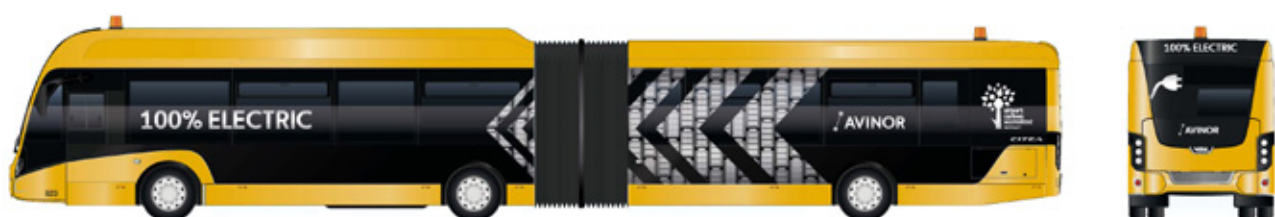
Oslo Airport's airside buses will appear as shown in the picture above. The buses are yellow due to airside visibility requirements.
