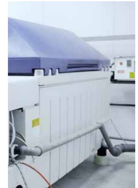
Corrosion Test - Salt-acetic fog chamber
