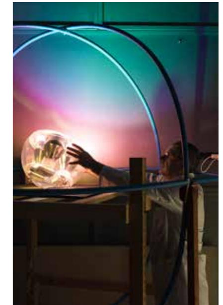
EMC Test - Triple Loop Antenna
