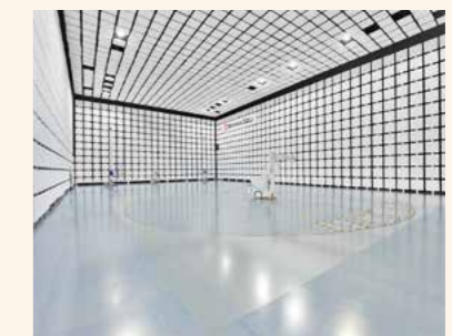
Anechoic Chamber at the Quality Center
