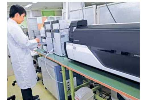
LCMS-8060 Ultra Fast Liquid Chromatograph Mass Spectrometer Using for Analyzing Hazardous Substances Adhering to the Surface of Microplastics
