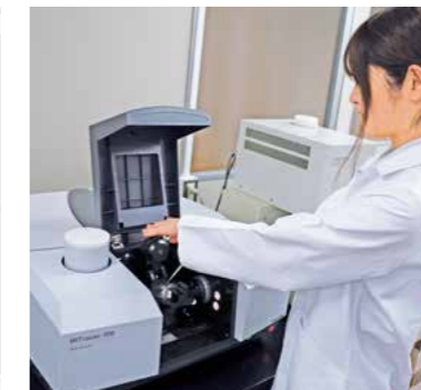
FTIR Spectrophotometer + Infrared Microscope Using for Identification of Microplastics
