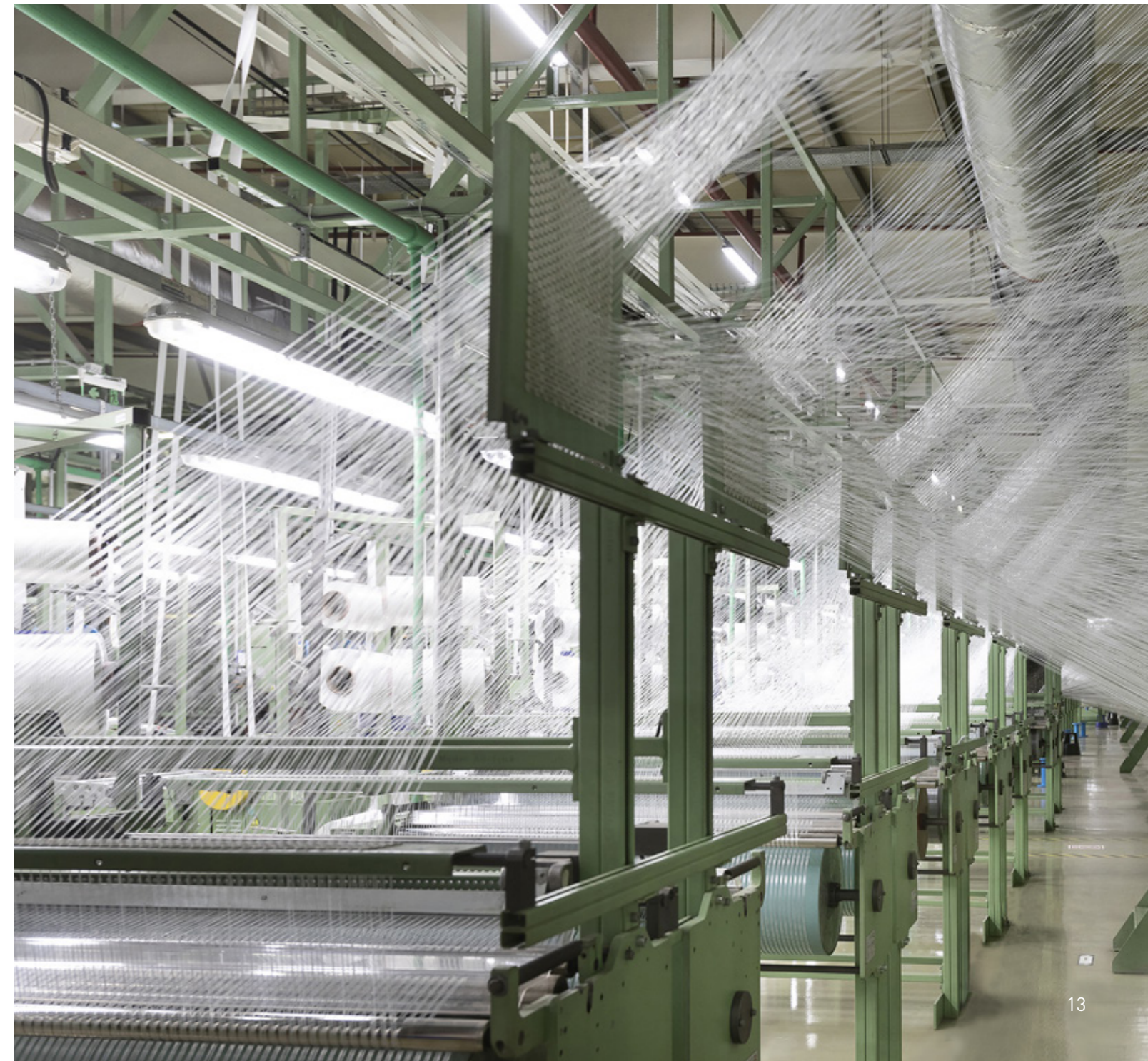
Image below: Seatbelt Webbing Process at Autoliv in Brasov, Romania
