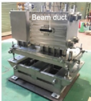
Figure 1. Exterior of the high-temperature superconducting electromagnet
