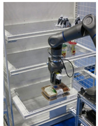
Holding a product using the suction pad unit
