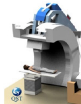
Figure 3. Ultra-compact heavy ion beam cancer treatment (rotating gantry) Provided by Kansai Photon Science Institute, National Institutes for Quantum and Radiological Science and Technology
