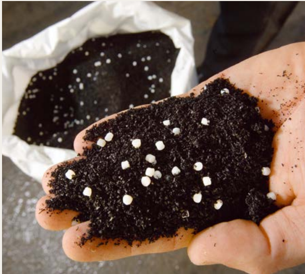
VESTENAMER® (white granulate) from Evonik facilitates efficient reprocessing of rubber (black granulate).
