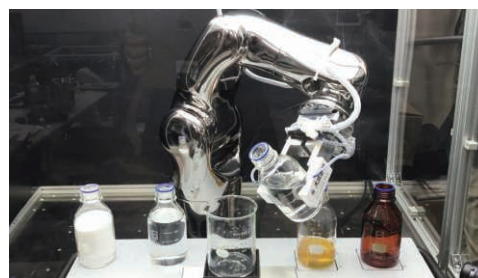
Liquid weighing operation using a force-tactile transmission type remote control system equipped with AI
