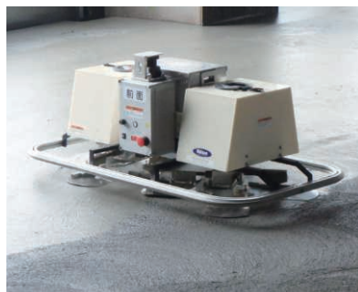
Concrete floor finishing robot T-iROBO® Slab Finisher
