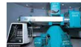
Centrifugal model experiment of foundation for offshore wind power
