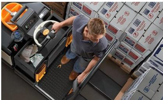
Double center rider electric pallet jack
