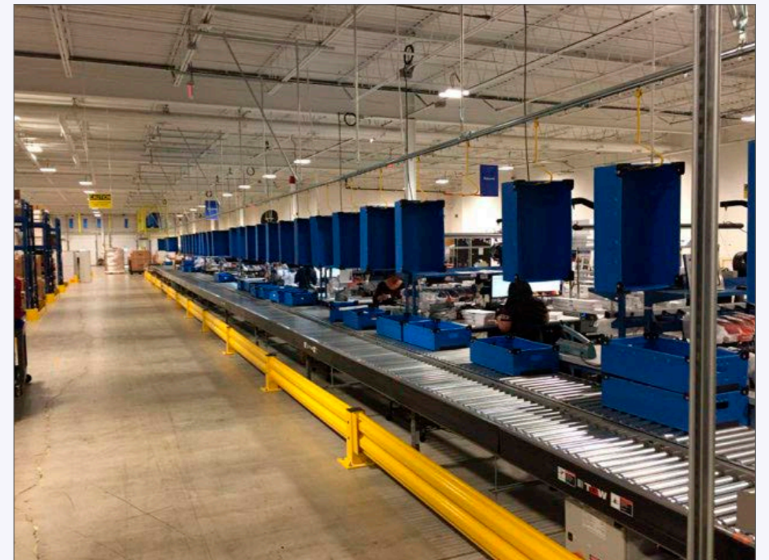
Process efficiencies at the Auburn distribution center include an overhead tote conveyor, which keeps walkways clear and safe while preventing wasted effort
